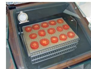
Turn one of the latches (located on the right hand side which seals the glass door) on the **SUN OVEN®** inward and set the glass on top leaving a gap between the black gasket and the glass to allow moisture to escape.
